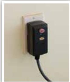
The pump operates on 115 volts AC, 50/60 cycle and draws 1.50 amps. The GFI must be plugged into a 3 wire, *grounded*, 115 volt outlet. The ground path ***must not*** be defeated by the use of a 2 wire cord, a 3 wire to 2 wire adaptor, or the removal of the ground pin.
